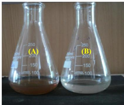
Figure 1 Colour changes after (AgNPs) the process of reduction of Ag + to Ag nanoparticles and control (AgNO 3 )
