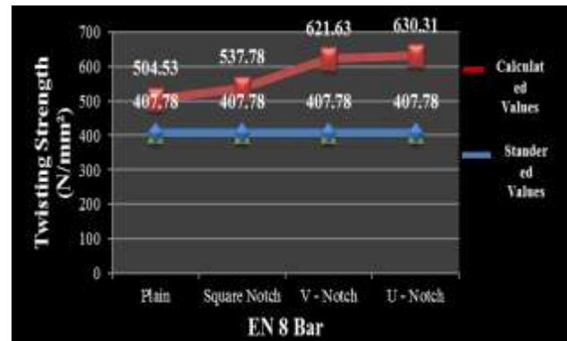
Fig. 11: Notch Effect on Twisting Strength of Bar (12 mm dia.)
