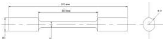
**Fig. 2: Specimen without Notch (9mm Dia.)**
