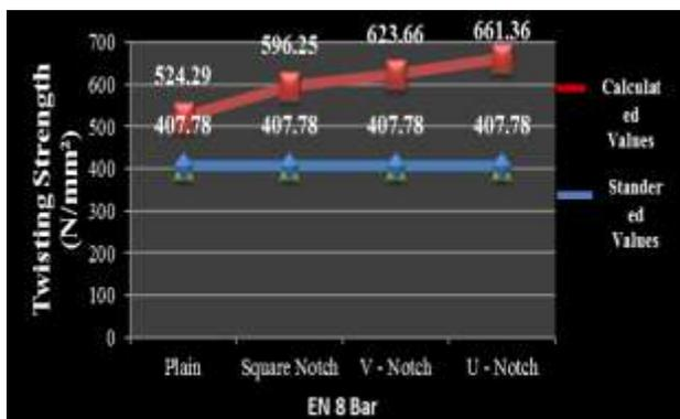
Fig. 10: Notch Effect on Twisting Strength of Bar (9 mm dia.)
