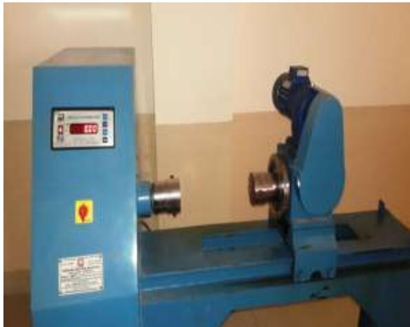
**Fig. 1: Experimental setup of Torsion Testing Machine**
