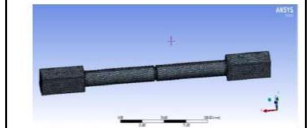
Figure 26: Mesh (Bar with U Notch 3mm depth)
