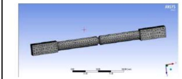
Figure 24: Mesh (Bar with V Notch 3mm depth)
