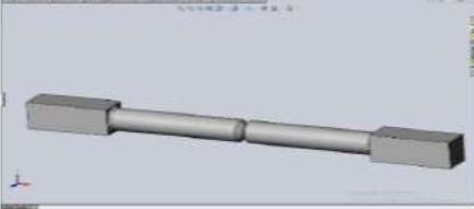
Figure 16: Bar with V Notch 3mm depth
