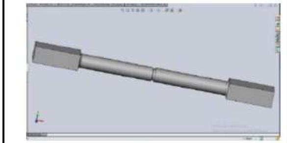
Figure 18: Bar with U Notch 3mm depth
