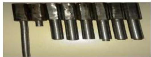
Figure 27: Specimens after Twisting Testing from Torsion Testing Machine
