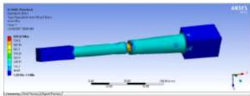
Figure 30: ANSYS Analysis of Bar with Square Notch 3mm Depth
