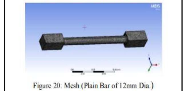
Figure 20: Mesh (Plain Bar of 12mm Dia.)
