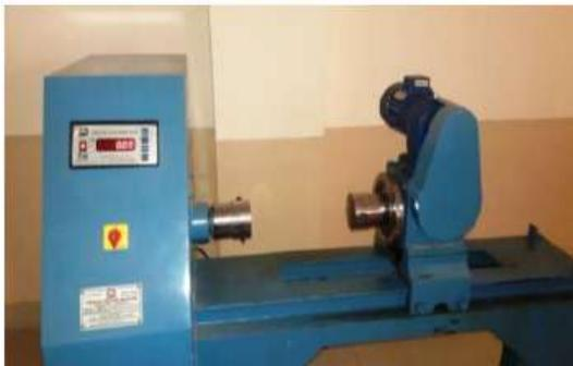
Figure 1: Experimental setup of Torsion Testing Machine
