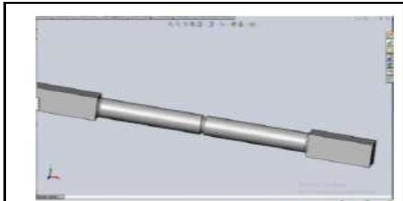
Figure 17: Bar with U Notch 1.5mm depth
