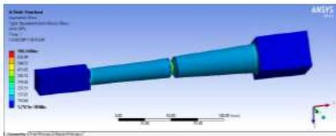
Figure 31: ANSYS Analysis of Bar with V Notch 3mm Depth
