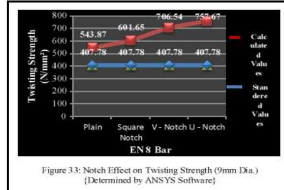
Figure 33: Notch Effect on Twisting Strength (9mm Dia.) {Determined by ANSYS Software}
