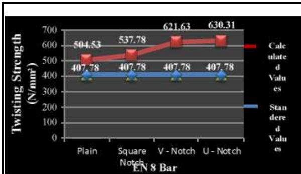
Figure 35: Notch Effect on Twisting Strength of Bar (12mm Dia.) (Determined by Torsion Testing Machine)
