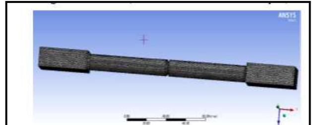
Figure 25: Mesh (Bar with U Notch 1.5mm depth)
